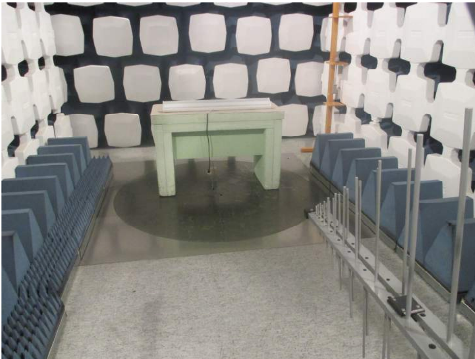
Figure 3: Radiated emission test
