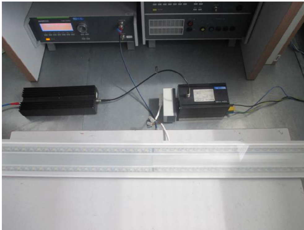
Figure 14: Immunity to conducted disturbances induced by RF fields
