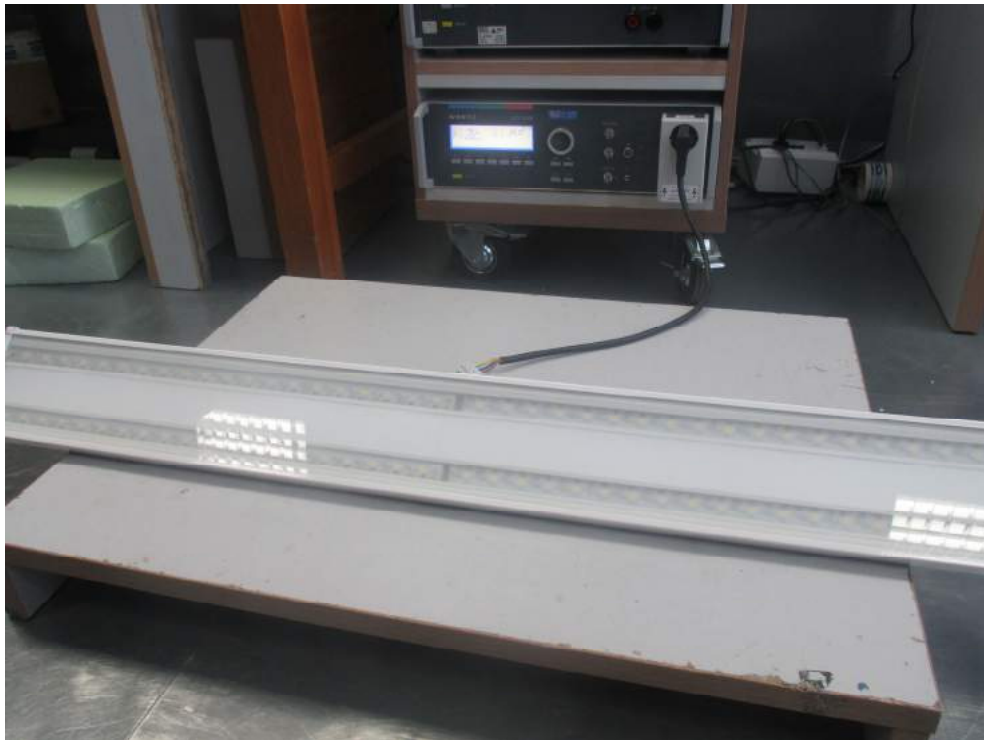
Figure 16: Voltage dips and short interruptions immunity test (DIP)
