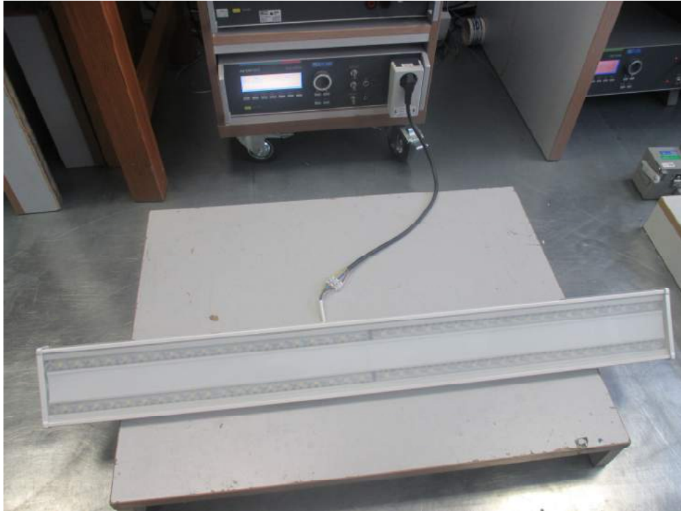
Figure 13: Fast transient / burst immunity test and surge immunity test
